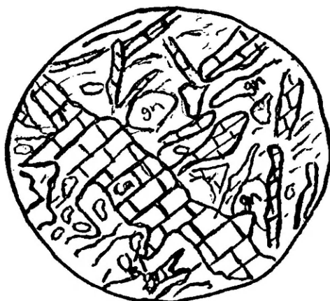
Fig. 36. Galena (gn) being replaced by calcite (cal) along fractures, 2381, (X8).
