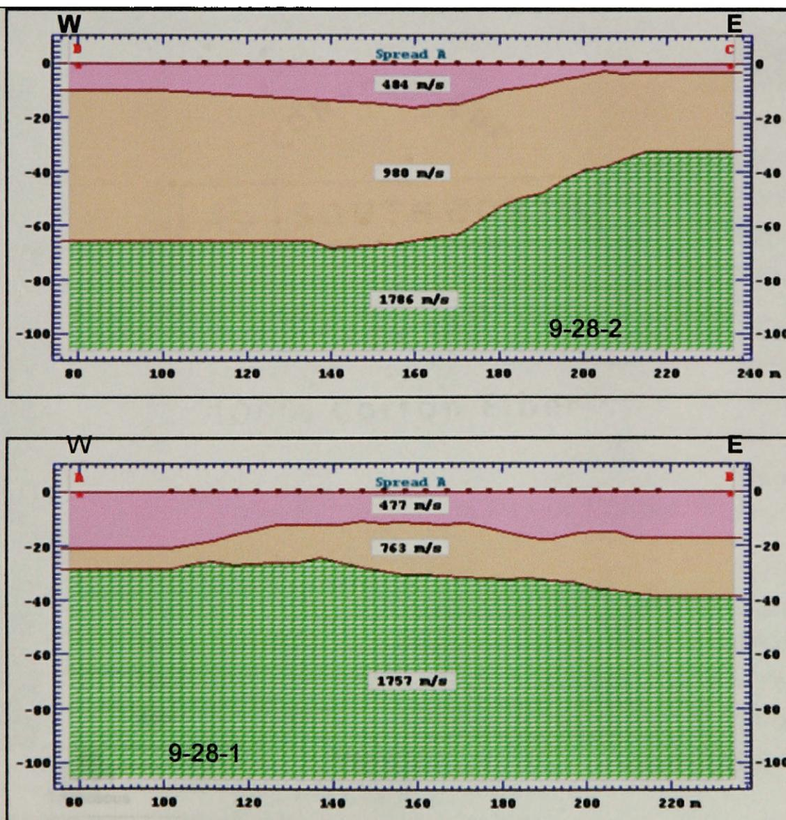
Figure. 8: Coberly gulch seismic profiles. 9-28-1 a (top), 9-28-2 (bottom). Note large displacement in top right this is interpreted as a small normal fault. Vertical axis is depth in meters. Horizontal is distance in meters.
