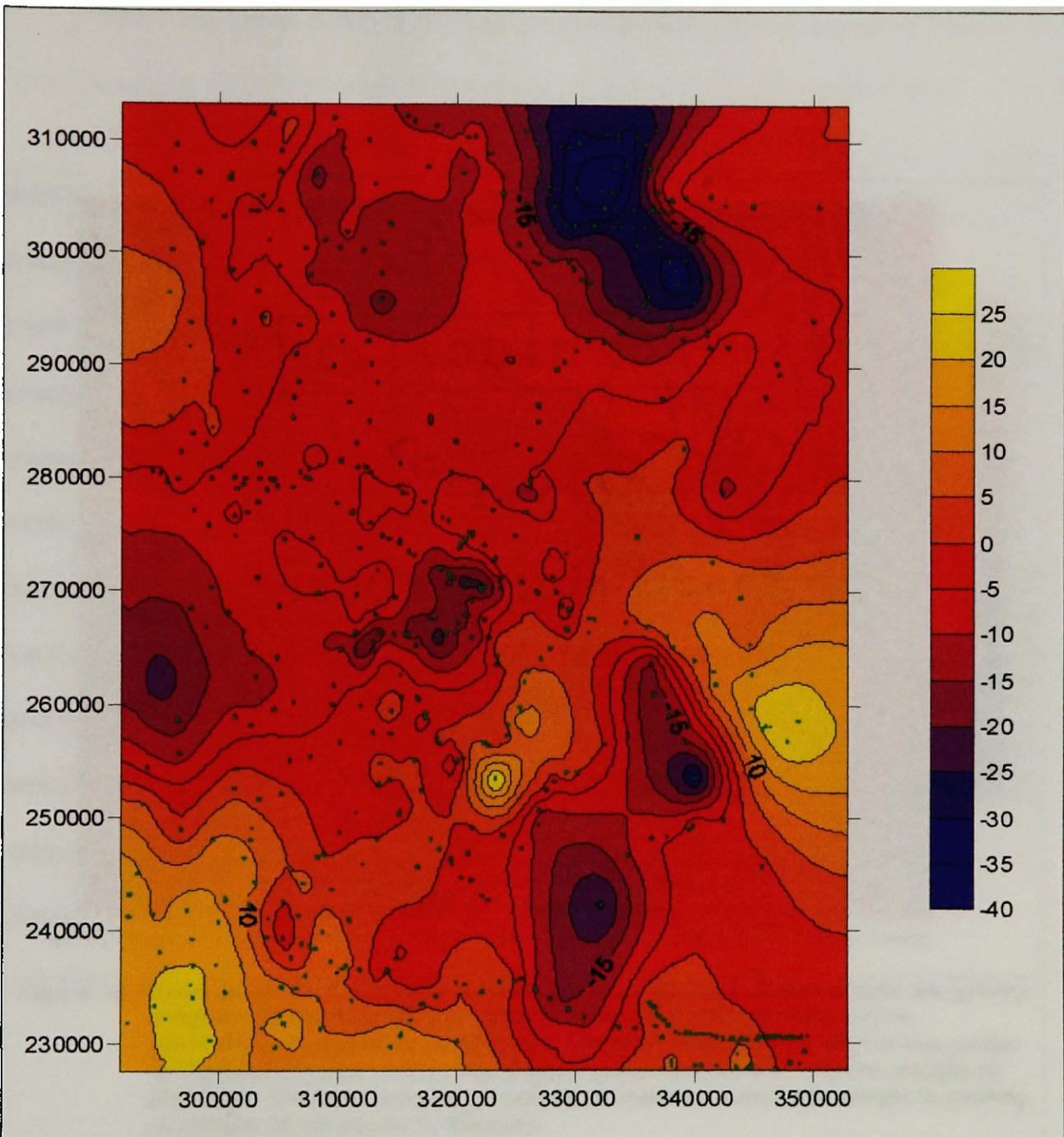
**Figure 15. Residual gravity signature (Figure 12 – Figure 13) shows shallow features such as sedimentary basins and shallow intrusive volcanic features. Vertical margin is northing in meters. Horizontal margin is easting in meters. Scale bar is in milligals.**
