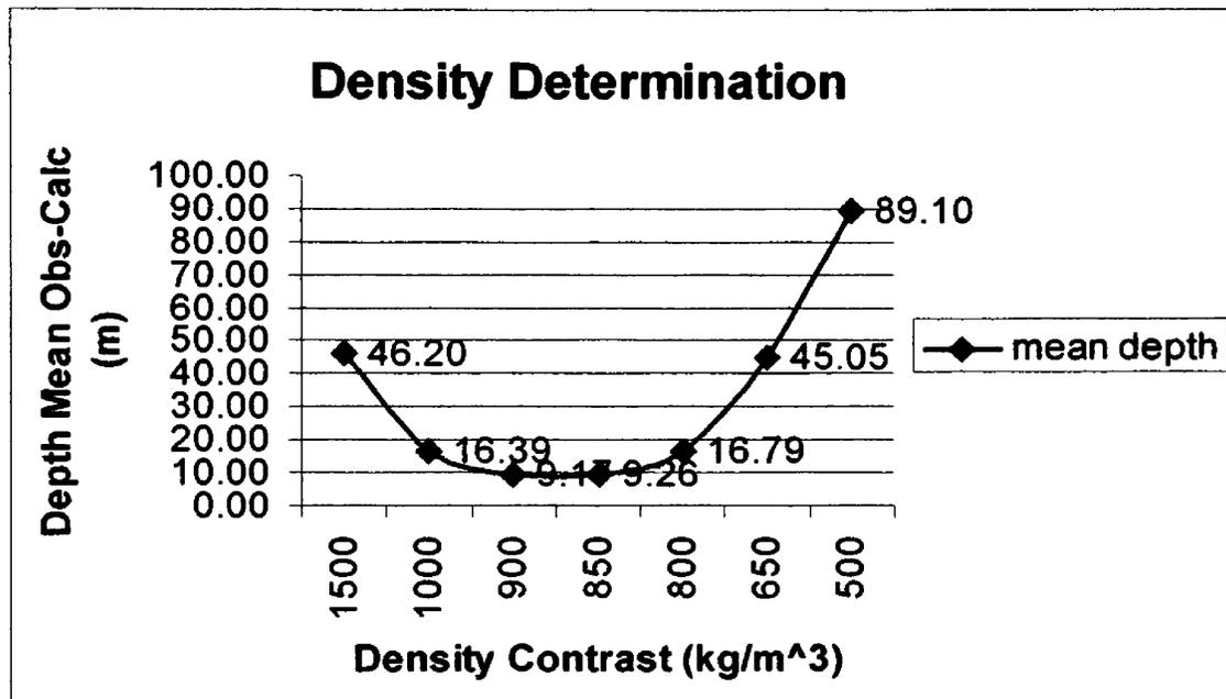
**Figure 18. Density contrast versus mean depth difference. The lower the difference between observed depth and depth calculated by the 2D sections the more accurately the model is depicting the basin, thus areas without the benefit of depth data. I chose a final density difference of 900 kg/m<sup>3</sup> for the basin based on the 2D model data.**
