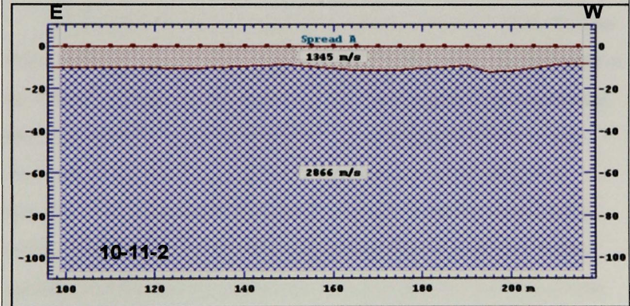
Figure 7. Dunkelberg ridge seismic profiles. 10-11-1 a (top), 10-11-2 b (bottom). Vertical axis is depth in meters. Horizontal axis is distance in meters with no vertical exaggeration
