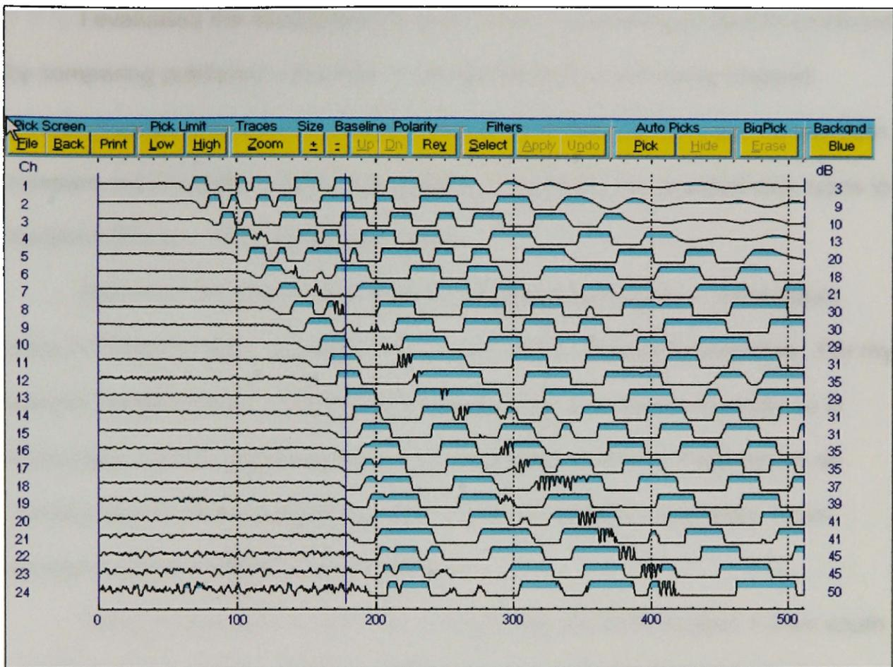
**Figure 5. Sample refraction trace display. Vertical axis on left is geophone number; on right is the decibel gain of the phone. Horizontal axis is time in ms.**
