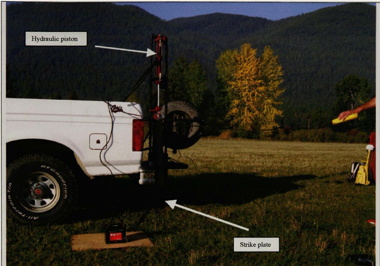
**Figure 4. Bison I Elastic wave generator. Note tail hitch mount and hydraulic hand operation. Strike plate is directly beneath the red piston. The inertial switch to the seismograph is attached to the strike plate**
