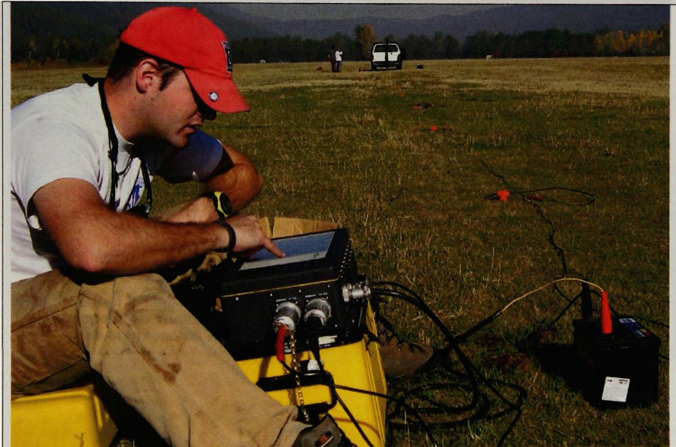
**Figure 3. Author operating the Geometric Smartseis 24 channel seismograph. Geophones (orange) and wave generator are in the background.**
