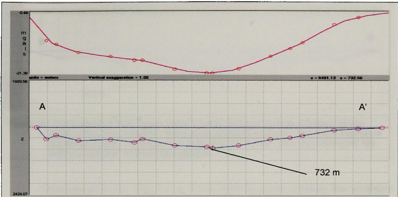
Figure 19. Cross section A-A'. Upper section is the modeled gravity anomaly for the basin in the lower section. Red points are known gravity. The lower section is the basin profile. The black line indicates the lowest point (in meters) on the bedrock surface for the cross section.
