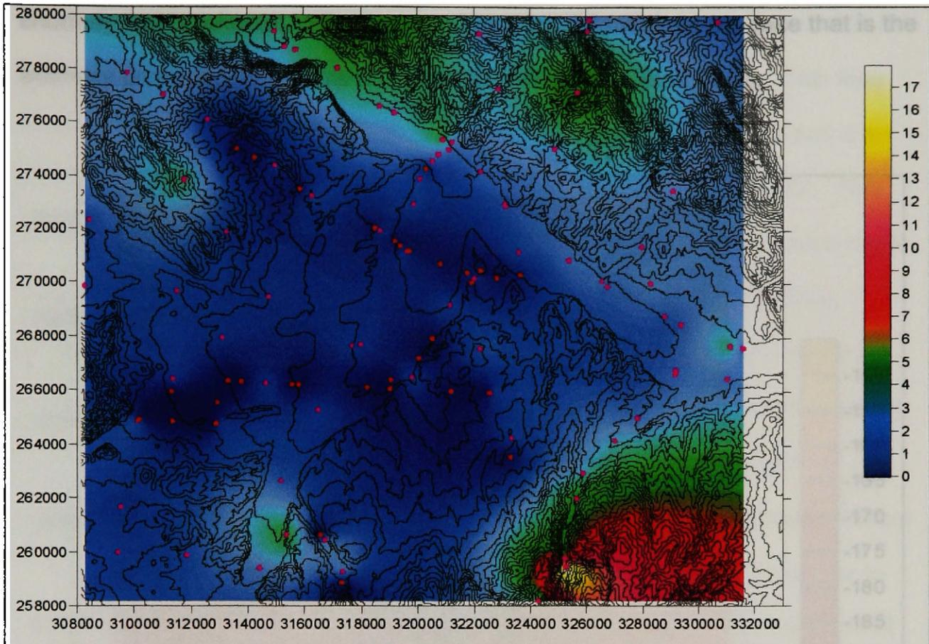
**Figure 12. Terrain corrections are in color. The black lines are elevation. Purple points are NDMC data. Red points are my data. Note the majority of my points have a correction less than 1 milligal. Color bar is the terrain correction in milligals. Vertical scale is northing. Horizontal scale is easting. Both are in Montana State plane.**
