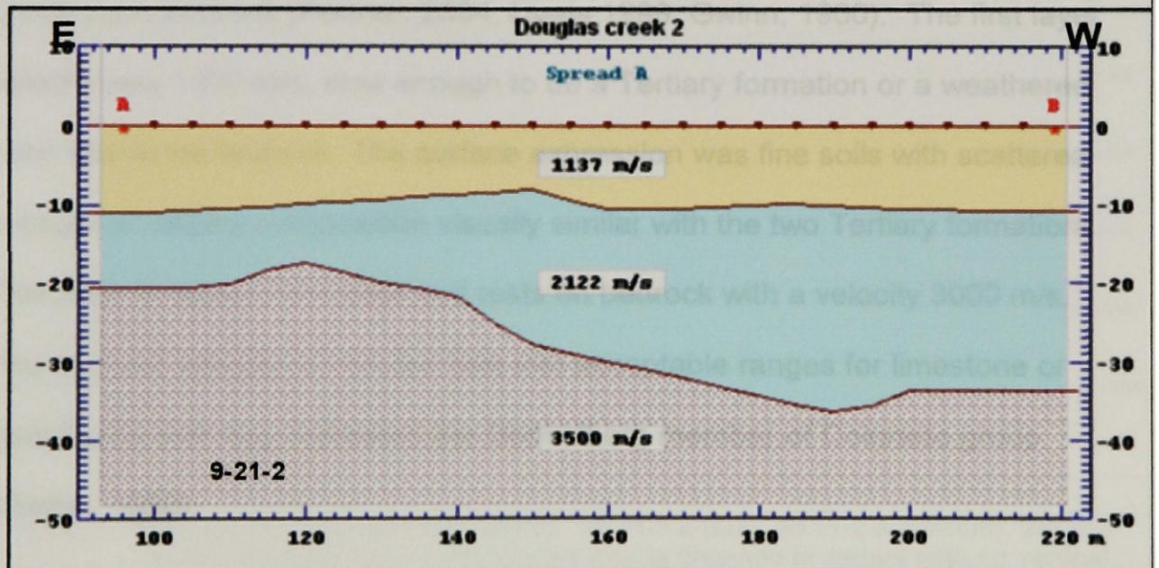
Figure 6. Douglas creek seismic profiles. 9-21-1 a (top). 9-21-2 b (bottom). Vertical axis is depth in meters. Horizontal is distance in meters. Vertical exaggeration is 1:2
