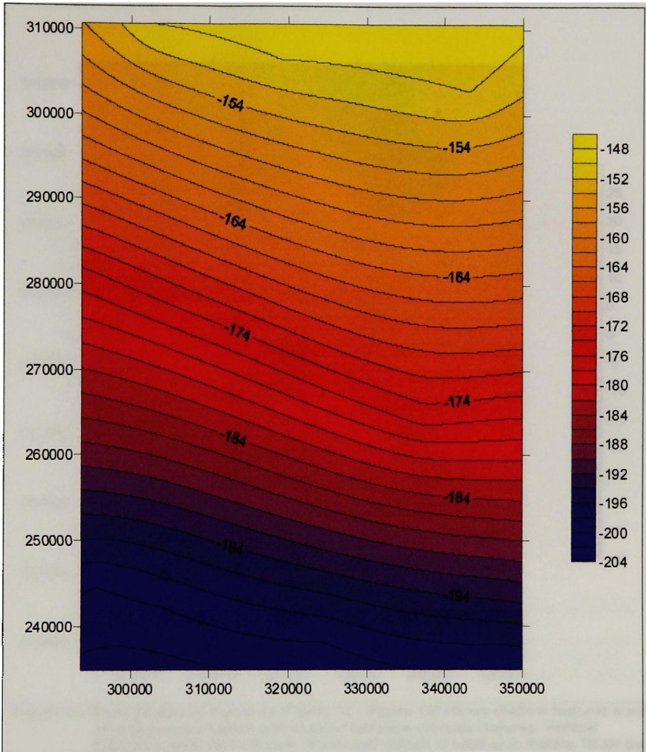
**Figure 14. Regional gravity signature caused by deep crust/mantle contacts and regional crustal features. Vertical axis is northing in meters. Horizontal axis is easting in meters. Scale bar is in milligals.**
