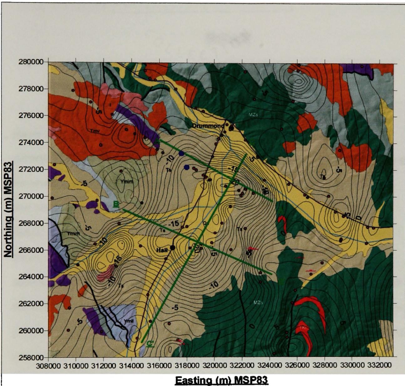
**Fig 2:** General geologic map of the Flint Creek basin. Contours are residual gravity. Red dots are gravity stations. Green lines are 2D cross sections. Black lines are faults. Pink lines are seismic refraction lines, and blue circles represent wells, which penetrate to bedrock. (Lewis, 1998 1:250k Butte Quadrangle)
