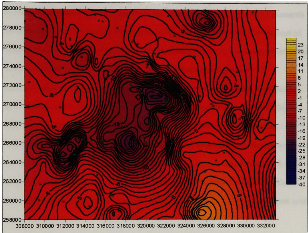
**Figure 16. Close up of the Flint Creek basin's gravity signature. Green points are gravity stations; blues indicate low gravity; Reds and yellows are positive anomalies. Scale bar is in milligals. The east west relative high in the center of the basin is due to the lack of gravity stations on the western margin of the basin. Vertical margin is northing in meters. Horizontal margin is easting in meters. Scale bar is in Milligals.**
