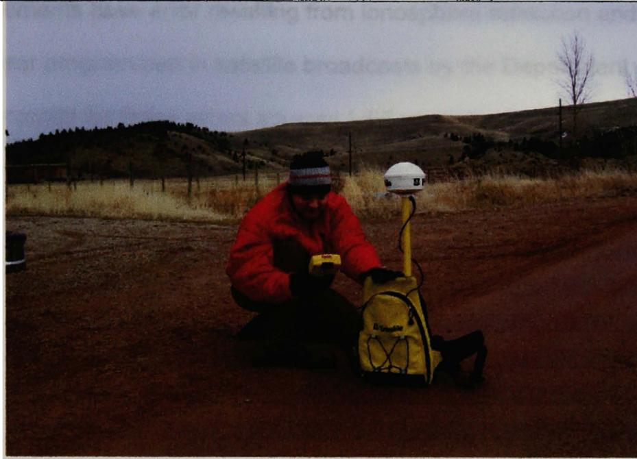
**Figure 9. Author operating the Trimble XRS PRO GPS system**
