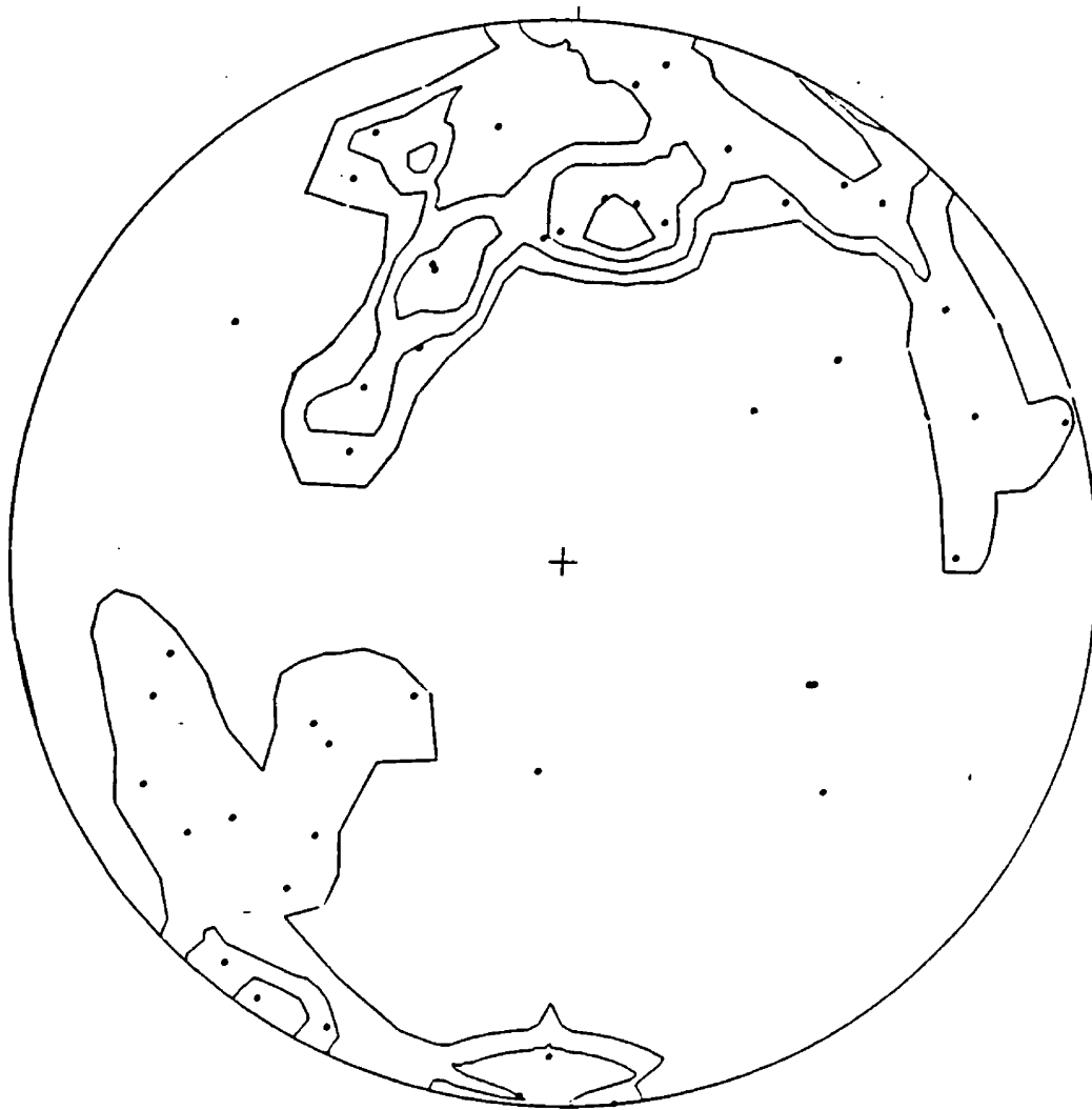
Figure 33c. Pi diagram of poles to foliation, Domain 18. Lower hemisphere equal-area projection. n=45 . Contours 2-4-6-7-9% per 1% area. Plot indicates poorly developed fold girdle plunging moderately to the southeast.
