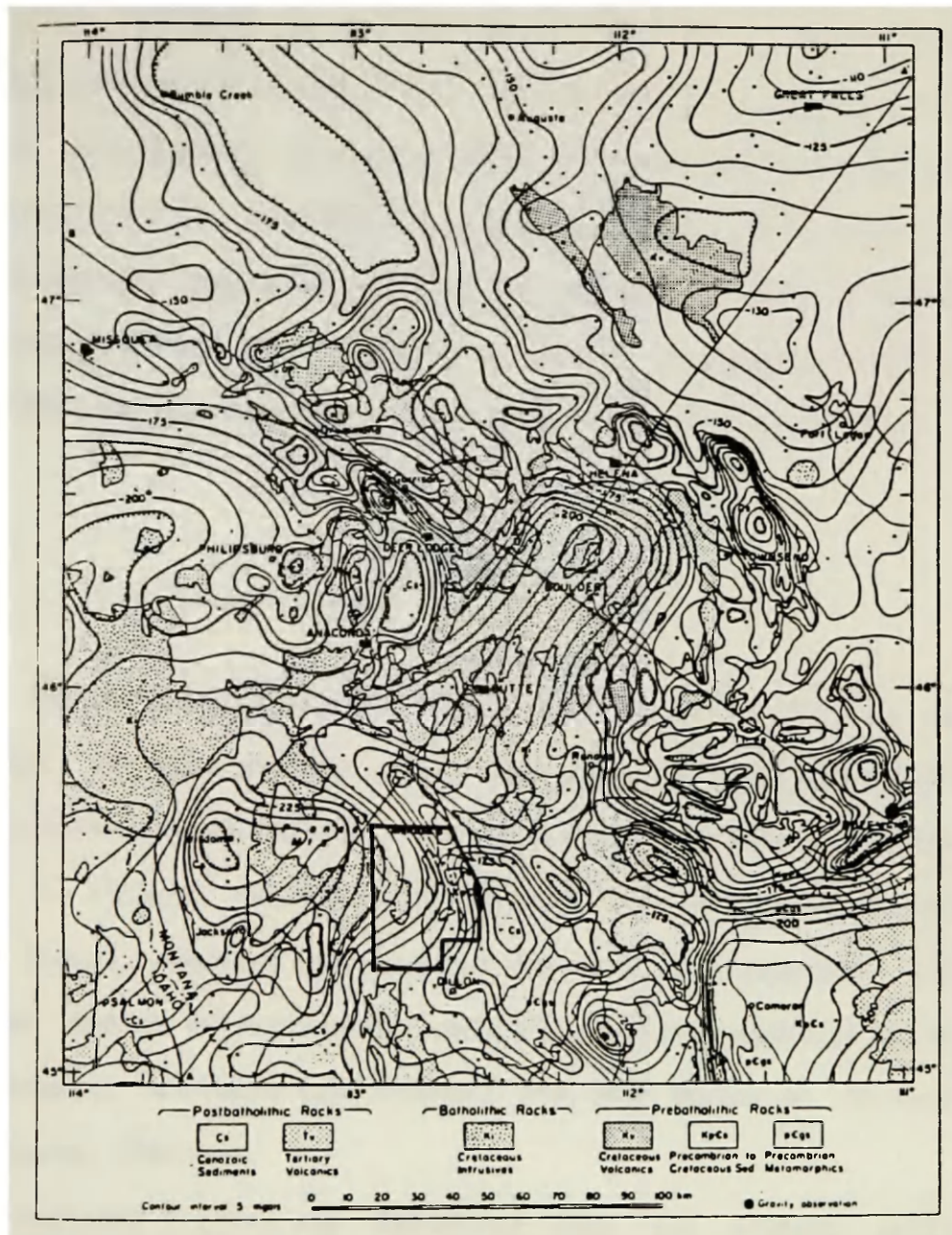
Figure 16. Simple Bouguer gravity anomalies and generalized geologic map of the Boulder batholith area. Dark box indicates boundary of present study area.
