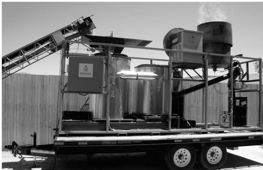
The operational dry weight feedstock throughputs of the two systems have been estimated by the manufacturers to be  $700 \text{ kg h}^{-1}$  and  $225 \text{ kg h}^{-1}$ , respectively. Biochar yields by mass are reported as between 5% and 25% for the TEA system and up to 24% for the BSI system, with the balance going to producer gas and a small fraction of ash and tar byproducts.
