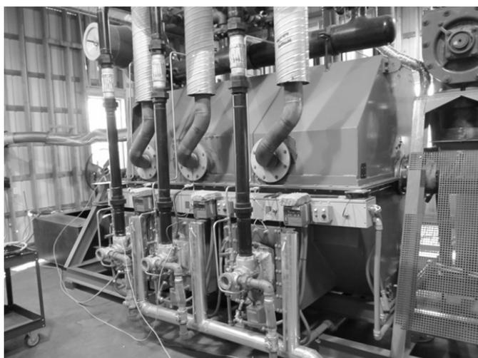
**Figure 2.** The Biochar Systems Incorporated (BSI), pyrolysis system Beta model used in this study. The unit used in this study was fitted with a thermal oxidizer (not shown), which replaces the open flare shown on the right. Photo: BSI.
