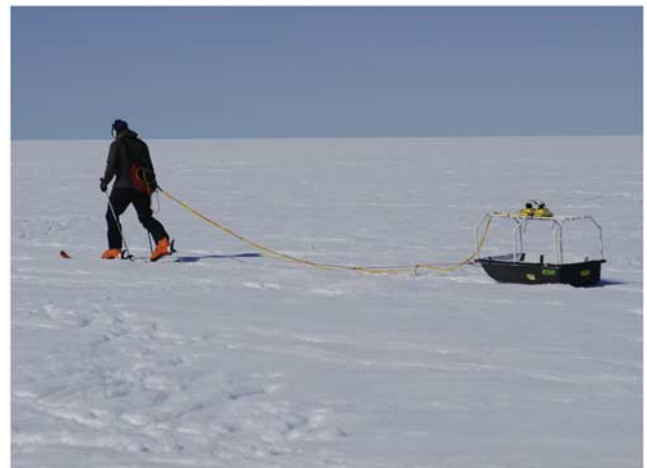
Figure 7. Sled and operator in the configuration for acquiring multioffset GPR data with the 1000 MHz antennas suspended 0.70 m above the snow surface.
