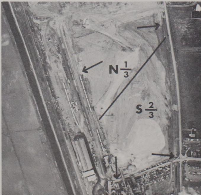
FIGURE 1. Photograph of Hoerner-Waldorf chip pile showing north one-third and south two-thirds. The arrows indicate target positions.
