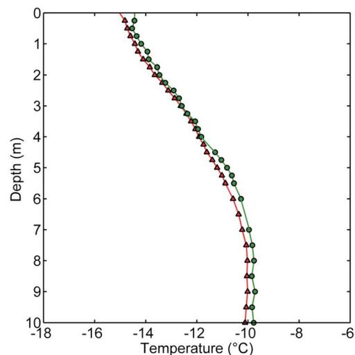
**Figure 2.** Temperature profile repeatability. Data are from two thermistor strings installed 10 m apart at site T1 and show a snapshot of temperatures on 5 May 2009. The two records agree within 0.5°C of each other. However, transient heating events due to localized meltwater infiltration and refreezing created marked differences between the two temperature profiles for periods of days to weeks.
