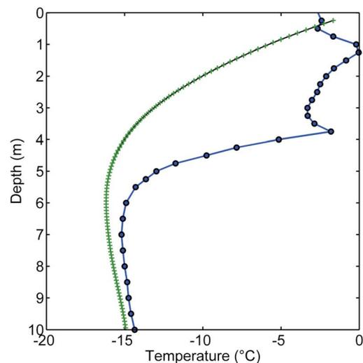
**Figure 4.** Infiltration heating event at site T3 occurring at midnight on day 204, 2007 (late July). Dots mark the measured temperature profile, with heating events at about 1.5 and 4 m depth. Crosses show the conductively modeled temperature profile based on measured air temperatures as the surface boundary condition.
