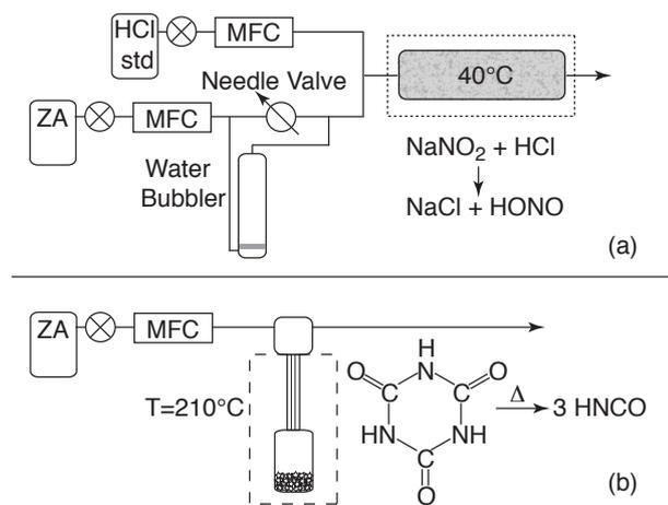
**Fig. 2.** Systems used to produce dilute streams of HCl and HNO<sub>2</sub> (a), and HNCO (b) for the calibration of the NI-PT-CIMS instrument.
