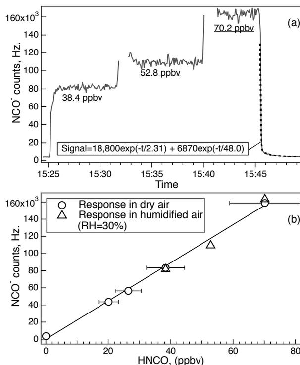
**Fig. 7.** Panel (a) shows the response of the NI-PT-CIMS to the HNCO standard (gray line), introduced through the entire inlet. A double exponential fit to the HNCO signal when the standard was removed (dashed line) is also shown. Panel (b) shows the results of HNCO calibrations under dry (circles) and 30% humidity (triangles).
