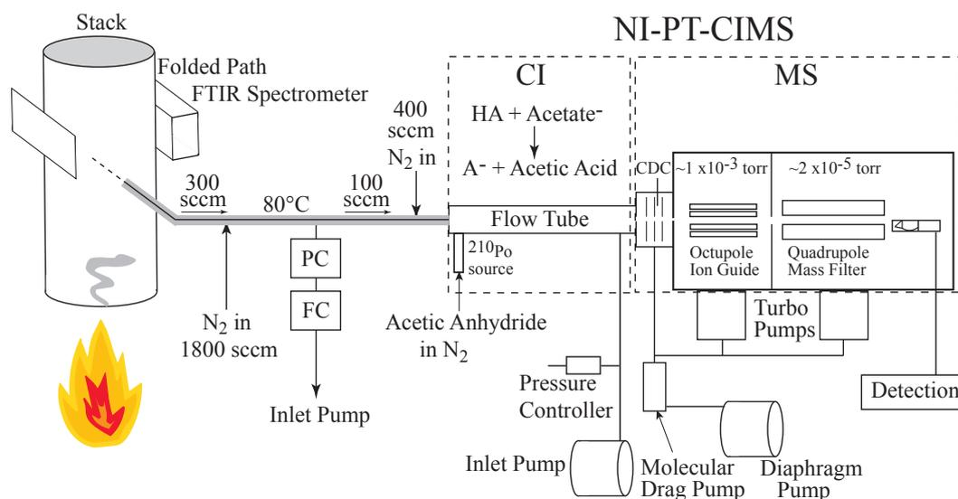
**Fig. 1.** Diagram (not to scale) of the NI-PT-CIMS and associated inlet system used for sampling the biomass burning experiments. The gray shading on the inlet line denotes the part that was thermo-stated at 80 °C.
