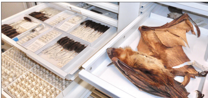
ABOVE: Two drawer sizes, optional middle posts, and tracks spaced every inch allow customization to perfectly fit specimens large and small.
