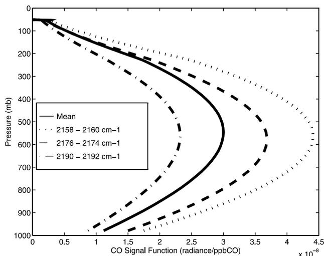
**Figure 2.** CO sensitivity functions ( $SF_{CO}$ ) for a constant CO mixing ratio in the troposphere, AFGL standard atmosphere, and surface air thermal contrast of 5 K.  $SF_{CO}$  for CO lines at 2158.2997, 2176.284, and 2190.018  $\text{cm}^{-1}$  are shown along with the mean  $SF_{CO}$  for the 17 CO lines in the 2135–2200  $\text{cm}^{-1}$  spectral region.  $SF_{CO}$  were calculated for the nearest SHIS frequencies using the method of McMillan et al. [1997].
