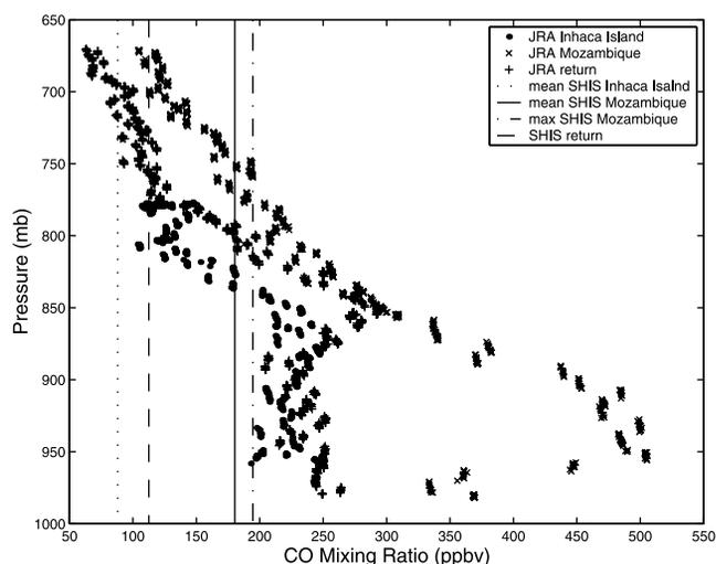
**Figure 10.** The comparison of JRA CO in situ CO profiles and SHIS CO retrievals presented here is for qualitative purposes. Note the larger CO values seen by JRA at all levels over the *river of smoke* in Mozambique (X's) as compared to the two profiles acquired on the other side of the westerly wave. The SHIS retrievals show the same spatial variations.
