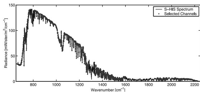
**Figure 1.** This sample full SHIS spectrum from 7 September 2000 shows the locations of channels used for the retrieval of atmospheric temperature and moisture profiles as well as surface temperature. The spectral region used for the CO retrieval appears at the right end centered near  $2142\text{ cm}^{-1}$ .
