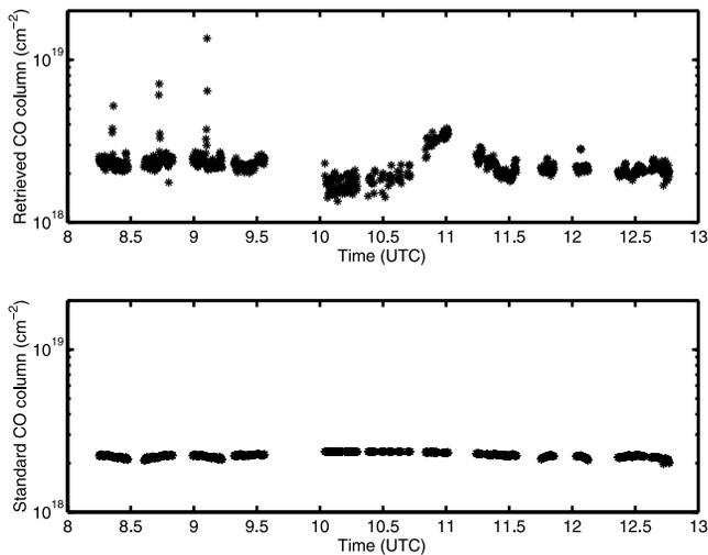
**Figure 6.** The top panel depicts retrievals of total tropospheric column CO from 742 cloud-free averages of 12 SHIS spectra acquired on 7 September 2000 during SAFARI 2000. The bottom panel shows the expected spatial variation in total tropospheric CO column due to topographic and aircraft flight altitude variations. The dissimilarity between these two plots implies substantial real variations in tropospheric column CO.
