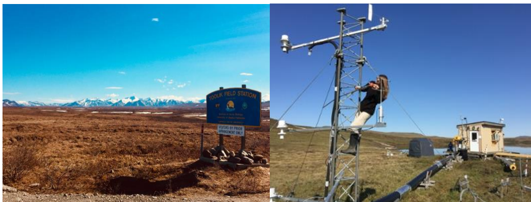
Figure 1. Left: Photo of the Toolik Field Station in the north slope of Alaska. Right: Photo of UM graduate student Catie Wielgasz replacing sampling inlet filter during the field campaign at the Toolik Field Station.
