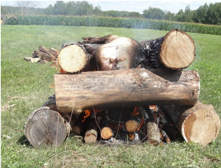
Figure 2. The lattice structure of the fires, with thermocouple wires visible.
