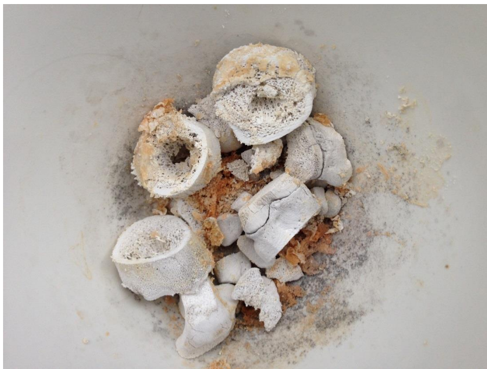
Figure 7. Sample T-4 after burning in muffle furnace at 700°C.
