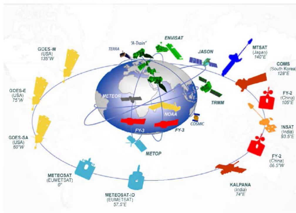
Figure 4. Schematic of the space-based Global Observing System (GOS) as of about 2010.
