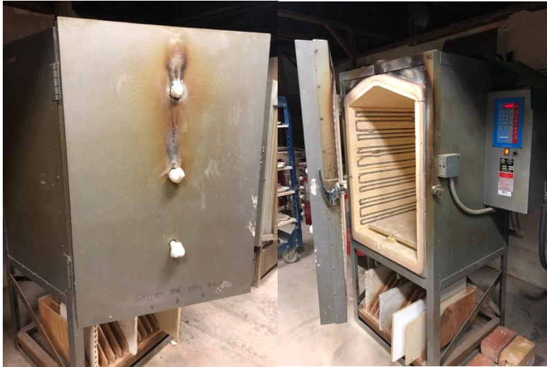
Figure 3c: Cross electric kiln. Left front view, and right-angled view of the inside and control panel
