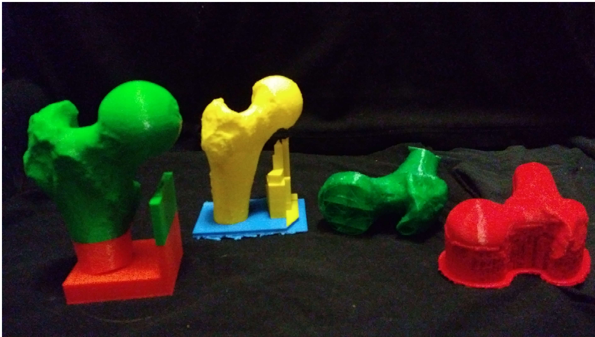
Image 6: This image constitutes of a group of 3D printed femurs. TX-16, on the far left and it shows that the print must be monitored every so often or else the printer might run out of filament and a change has to occur midprint. TX-17 in the middle left shows fall outs or little bumps on its surface because the extruder-point on the printer released too much filament at once, but it did not affect the overall measurements. TX-12 in the middle right shows what happens when the print gets too big for the printer. Lastly TX-14.2 is another print taken of TX-14 to show what can happen when the printer arithmetically inputs structures.
