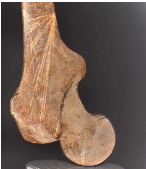
Image 5 (to the left): This image is of an original femur in the process of being scanned. This is a photograph taken by the NextEngine Scanner when it was in the middle of a 360-degree scan. This image shows more detail on it than we would see on a 3D copy of the bone. Note: reference Image 8 for what a 3D version of a proximal right femur looks like.
