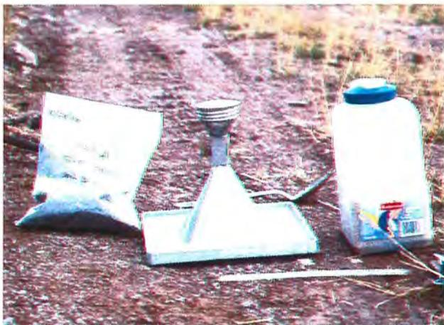
**Figure 3.4. Bulk density sample collected in the field.**
