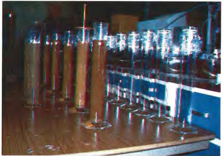
**Figure 3.19. Hydrometer analysis.**
