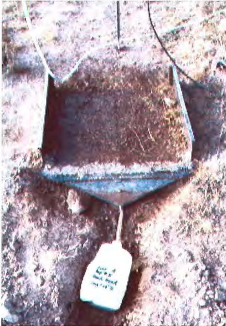
**Figure 3.11. Bentonite seal on triangle edge.**
