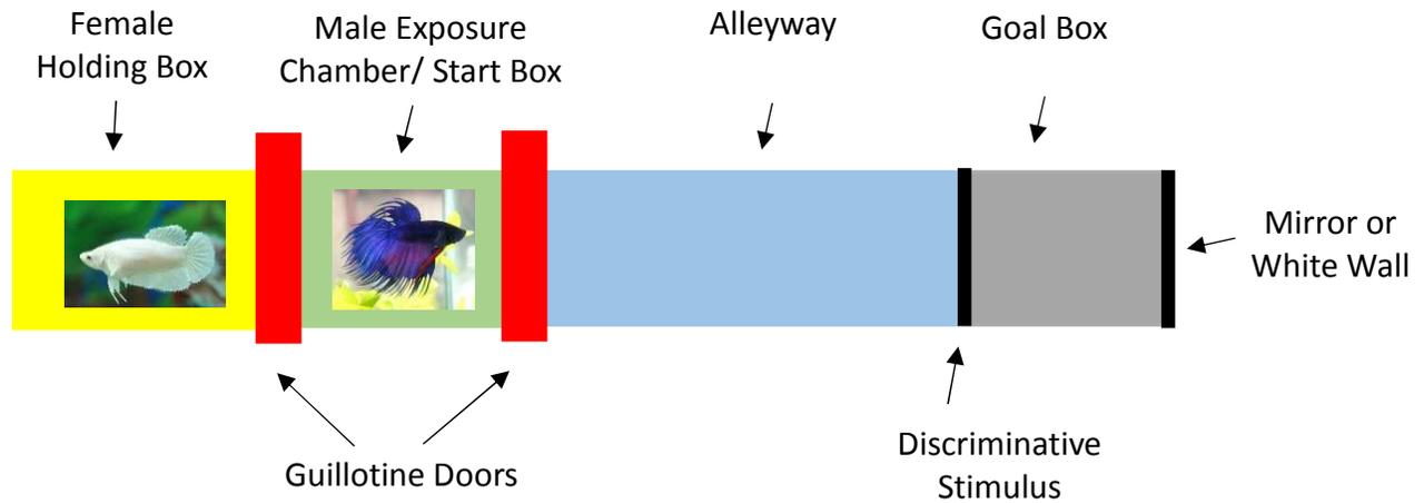
Figure 1. Diagram of the testing apparatus depicting the alleyway maze.
