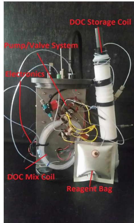
Figure 22 – DUCS mounted inside of SAMI instrumentation housing. A more detailed description of the plumbing and electrical design is shown in Appendix D.
