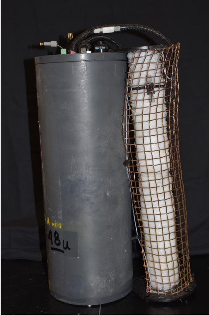
Figure 34 – Closed shell configuration of the DUCS. A copper mesh cage surrounds and protects the exposed black plastic covered sample coil. The electronics and plumbing (Fig. 22) are sealed airtight within the SAMI housing.
