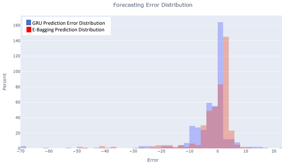
Figure 33: Prediction error distributions for the GRU model (blue histogram) and for E-Bagging (red histogram) for NY County; both are centered at zero. The latter has less variance.
