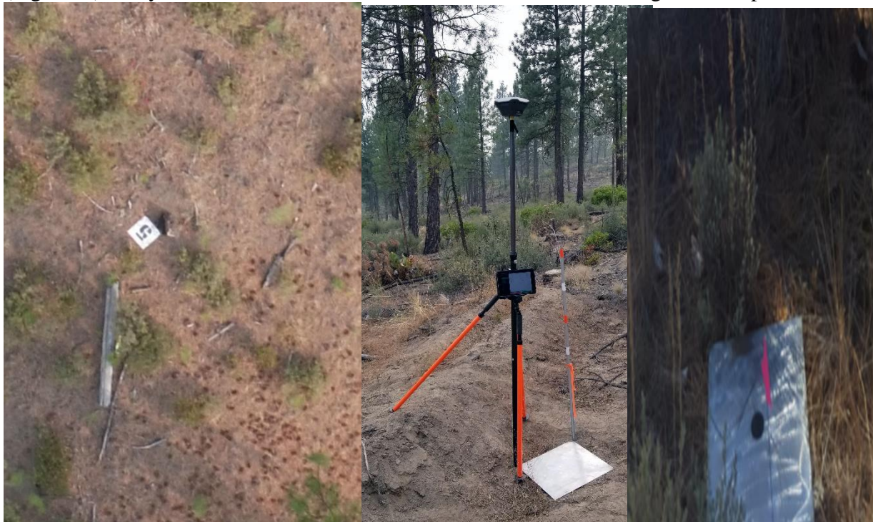
Figure 2. 2017 painted numbered GCP, 2018 GCP polished steel plate and 2019 GCP
