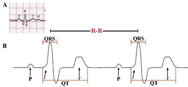
**Figure 1.** ECG waveform analysis is used for HRV measurement. RR intervals are the intervals between R waves within recorded QRS complexes. Figure adapted from Dong (2016).
