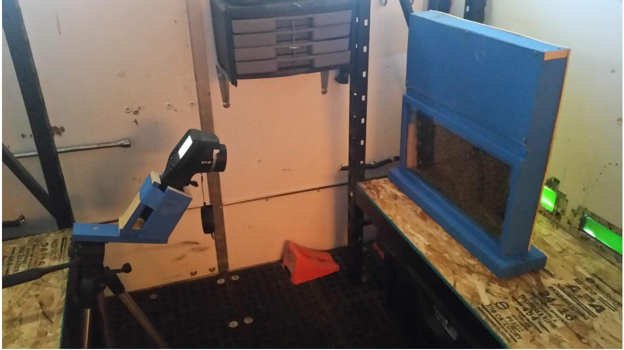
Supplementary figure 1. Observation hive for measurements of the proportion of nurse bees allocated to heater bee tasks.
