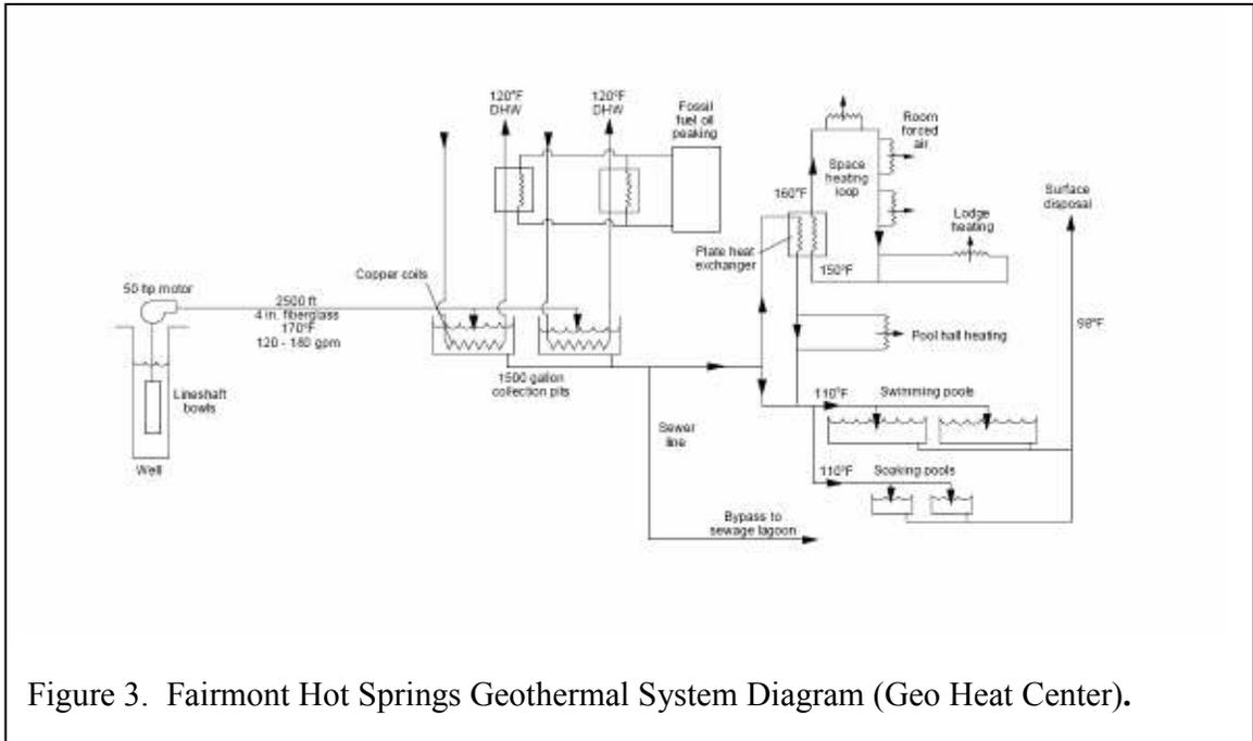
Figure 3. Fairmont Hot Springs Geothermal System Diagram (Geo Heat Center).
