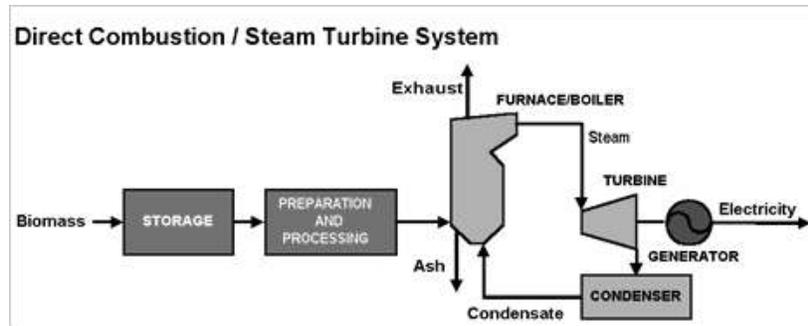
Figure 9. Electricity Generation from Biomass Combustion System (EERE).
