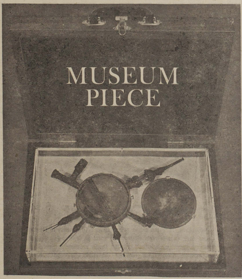
This cyclotron was built and operating by the fall of 1930 and reported at the Washington April Meeting (Phys. Rev. 37, 1707, 1931). The diameter of the chamber was about 5 inches. Placed between the 4-inch diameter poles of a magnet with a field of 12,700 gauss and 2,000 volts on its single dee, it produced 80,000 volt hydrogen molecule ions trapped and measured in a Faraday cage to which a measured and adequate decelerating voltage could be applied.
