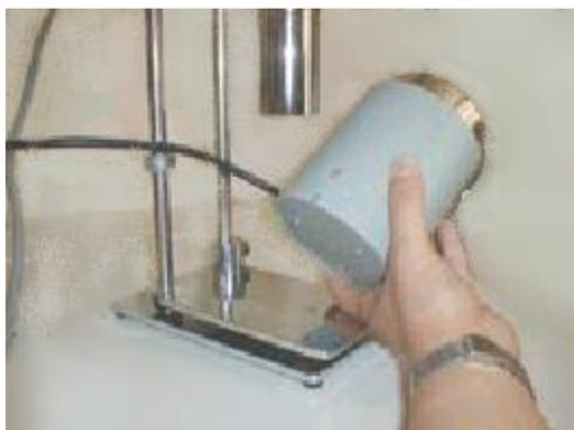
Pic 7. Put the cup assembly on stage.
