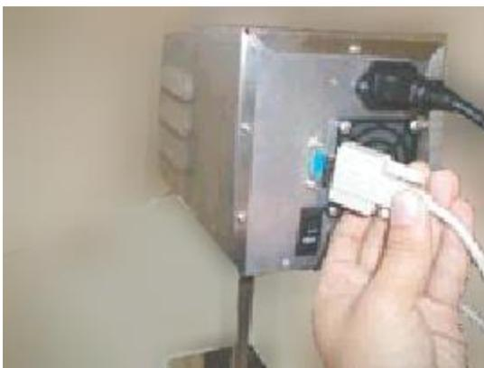
Pic 3. Plug in serial cable
