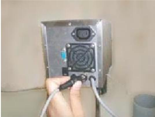
Pic. 1 Plug in temperature probe
