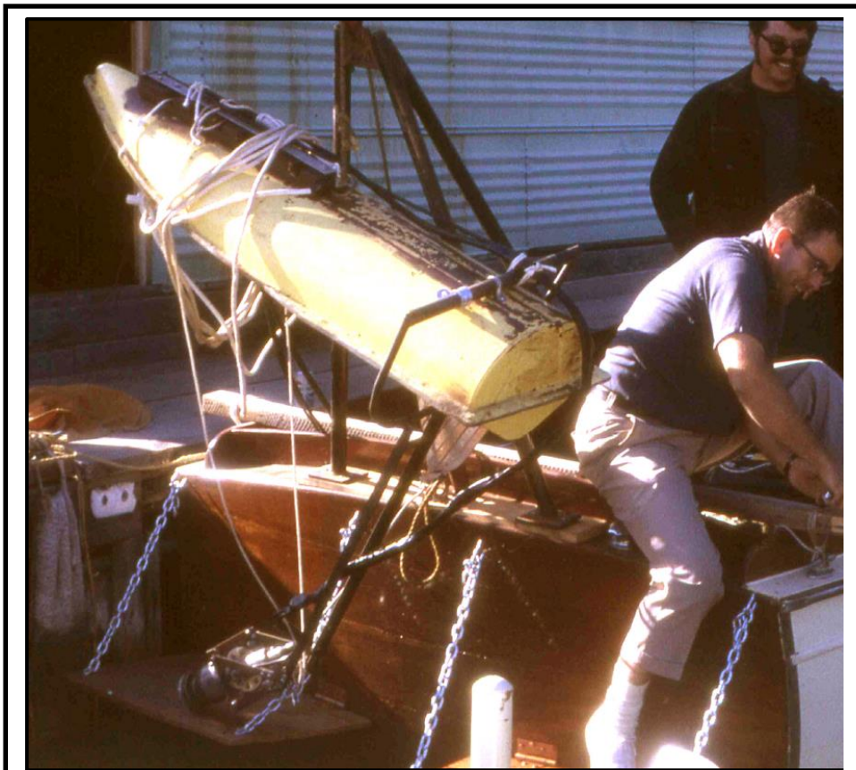
Figure 1. Air gun pontoon and suspension harness. The pontoon is the yellow item. The suspension harness is at the stern (right end) of the pontoon. The air gun itself is on the step on the stern of the survey boat in the lower left of the image. Original photograph courtesy of Richard Wold.
