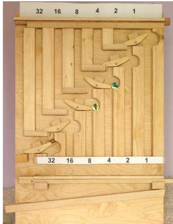
*Figure 10: Binary Addition Machine (Wandel)*
