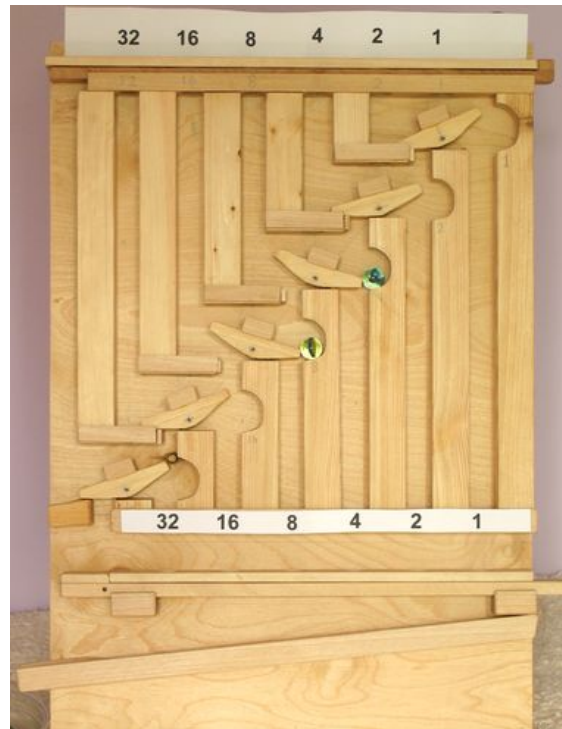
Figure 10: Binary Addition Machine (Wandel)
